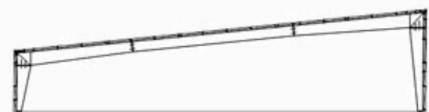
SINGLE SLOPE - RF (CLEAR SPAN)
