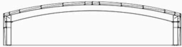
CURVE ROOF - RF (CLEAR SPAN)
